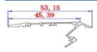
Surface-mounted LED strip profile with diffuser - 20x10mm - LED strip ≤ 15mm - 2 meters - 0.65mm - 21g/m
